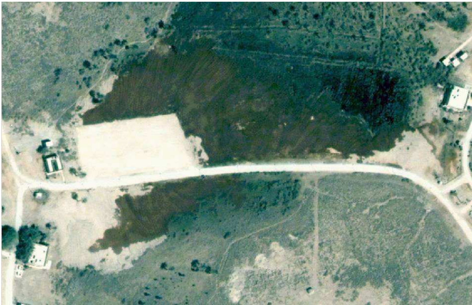
After construction of Landing Zone, prior to founding of Camp Babylon. Surface north and south of road has been bulldozed, graveled and oiled, 1 April 2003, Russell composite
